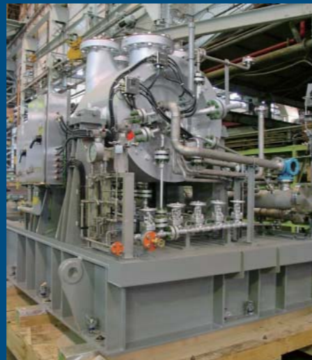
Gas Turbine driven compressor for natural gas service, CNL (Nigeria)
