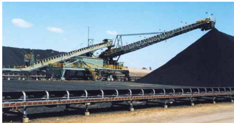
2,000 T/H linear slewing and luffing stacker
