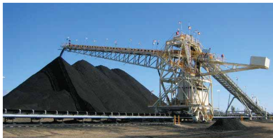
1,540 T/H linear luffing stacker
