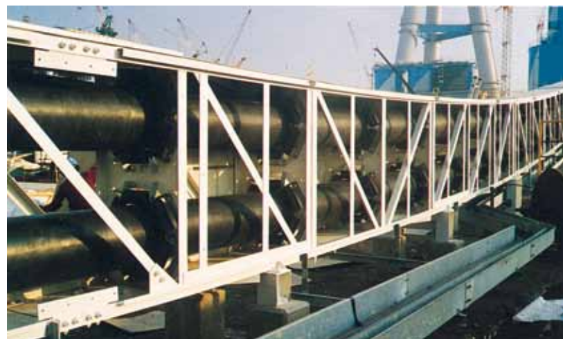
● Cross section of pipe conveyor (while being circularly enclosed)
