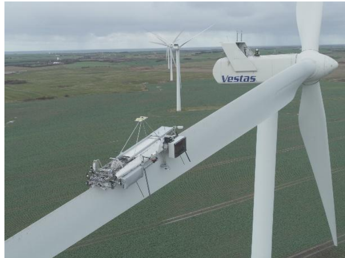
Leading-edge maintenance robot from BladeRobots
