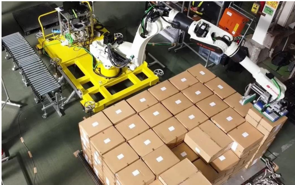
A scene from a pilot test for depalletizing goods from air cargo pallets
