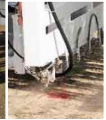
MINEDOG sensors (left). A map indicating detected mines in the test area (top right). The locations of detected mines are marked with red paint (bottom right).
