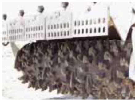
The MINEBULL's high-speed digging drum.
