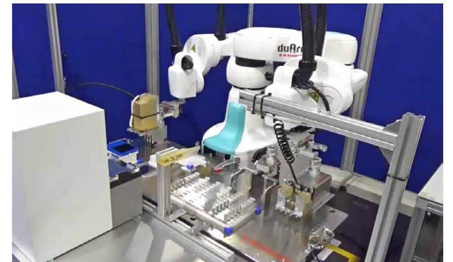
Building a system to reduce infection and increase the number of tests by automating the PCR test procedure.
