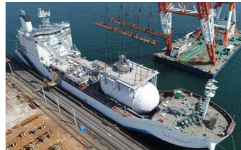
Installation of liquefied hydrogen storage tank for marine transport applications
