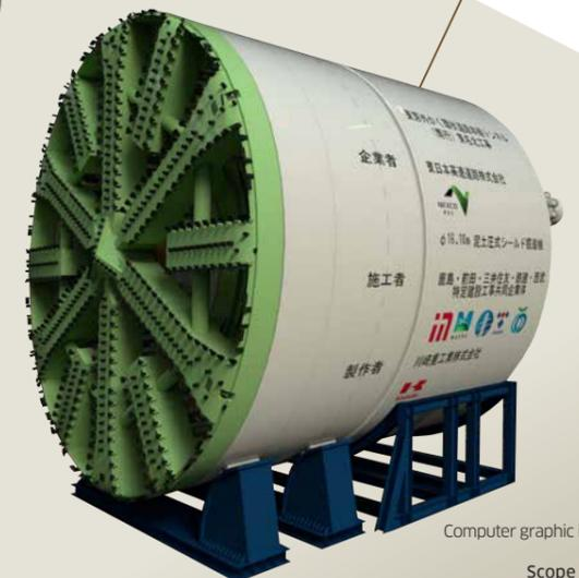
There are two main construction methods for underground tunnels: 1) the cut-and-cover tunneling method, in which the ground is excavated from the surface down, and 2) the shield tunneling method, in which a vertical shaft is excavated first (without further excavation from the surface) and then lateral excavation is performed from the vertical shaft.
