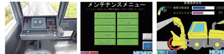
With the objective of achieving greater ease of operation and reducing labor, NICHIJO developed a monitoring system by which indoor staff are able to check, control, and record — in real time — information being transmitted from snowplows in the field. This system is also useful for responding expeditiously to failures and for recovery efforts.
