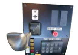
An intuitively-operable stick for controlling a snowplow which offers responsive maneuverability (for medium- to large-size snowplows). Before, users had to manipulate seven or eight levers in order to operate a snowplow.
