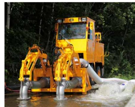
Grass cutters (upper photo) or emergency pumps for draining water from flooded areas (lower photo) are attachments which can be installed on the snowplow so that the machine can be used all year round, making it very cost-effective.
