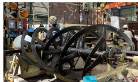
NICHIJO manufactures most of the parts for its snowplows in-house in order to meet customers' rigorous requirements. Photos show a snow-collecting auger (right) and a helical blade (above) being assembled (below).
