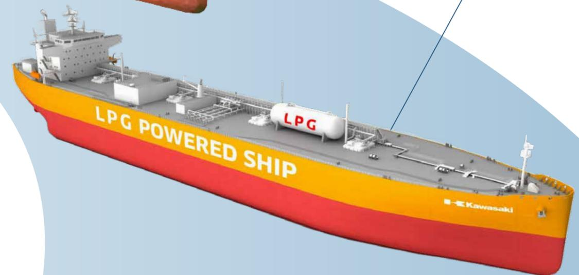
Building a vessel for transporting LPG or liquefied natural gas (LNG) requires sophisticated cryogenic technologies, which include material selection for the tanks, structural considerations, thermal insulation, and treatment of boil-off gas. Such expertise is considered one of the barometers for judging the level of a manufacturer's shipbuilding technology.
