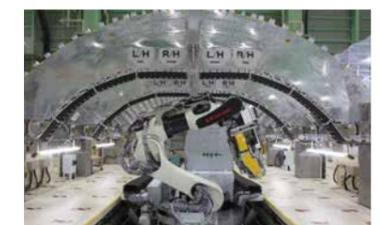
Tacking robot (robot for frame tacking)
