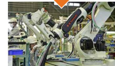
Components of the arm are added, beginning with the lowest section and, at the same time, the motor in the "joint" section of the arm is wired.
