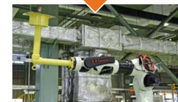
An inspection line for the finished robot: The L-shaped, yellow object is a weight used for inspection. Using this weight, each arm's range of motion, forward/backward, and up/down movements are checked.
