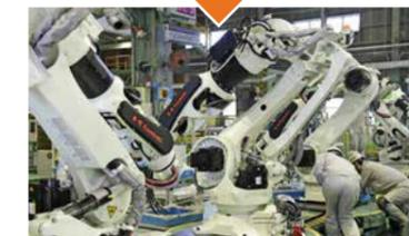
This is an extra-large, general-purpose robot with a payload capacity of 1,500 kg. Optional parts as needed for specific applications are attached to the tip of the arm.
