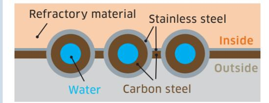
The U-KACC boiler adopts composite tubes for the water wall tubes to reduce sulfurization deoxidization corrosion in the high-temperature deoxidization zone. These tubes use high-strength carbon steel for the inner layer and corrosion-resistant stainless steel for the outer layer to prevent corrosion. As welding for composite tubes requires high skills, water wall of composite tube are manufactured at Kawasaki's Harima Works.
