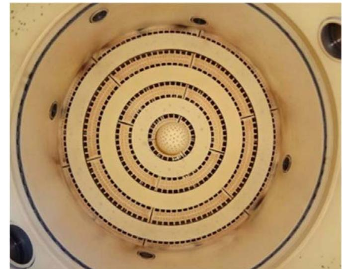
Combustor interior after 2h test
