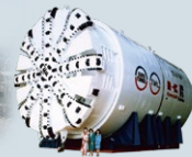
Tunnel boring machines used to excavate the Channel Tunnel, linking France and the United Kingdom
