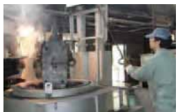
Before improvement: Heating incineration of resin
