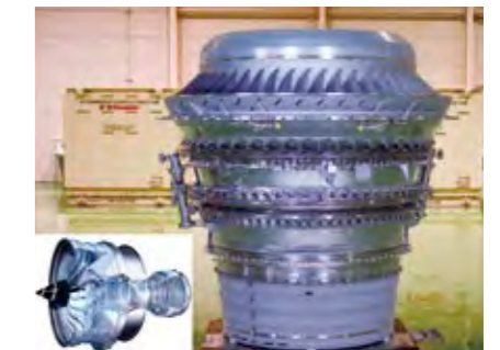
IPC module of Trent XWB turbopfan engine for Airbus A350XWB aircraft (IPC: Intermediate-pressure compressor)
