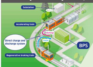
Introducing a cutting-edge high-performance battery with energy-saving potential and no electrical noise emissions
