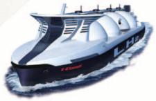
Hydrogen for use as an energy source will require handling in bulk. At the transport stage, a key question is how to carry the load more efficiently. Hydrogen, in its liquefied state, is extremely compact, taking up just one-eight-hundredth the volume of gas. The liquefied form is therefore the most optimal for transport and storage.
