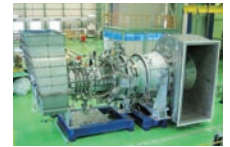
L30A gas turbine
