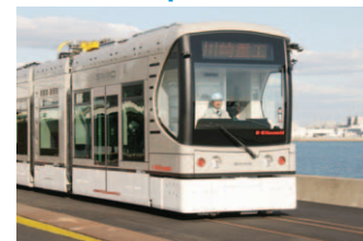
SWIMO: Low-Floor Battery-Powered Light Rail Vehicle (LRV)
