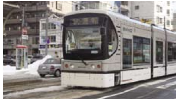
Test run without power supply from overhead lines in Sapporo
