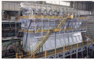
Two-cycle marine diesel engine
