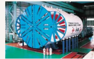
Detachable slurry triple station shield machine
