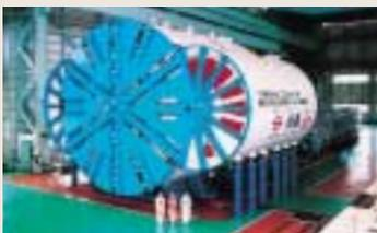
Detachable slurry triple station shield machine
