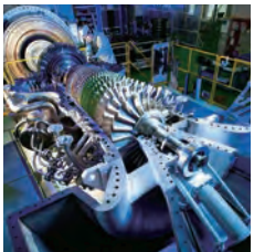
30 MW-class gas turbines
