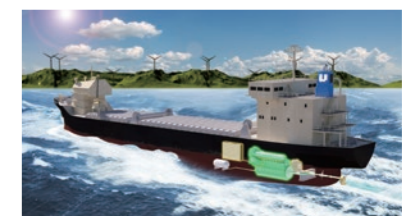
The Shimokita Maru equipped with a Kawasaki gas engine hybrid propulsion system
