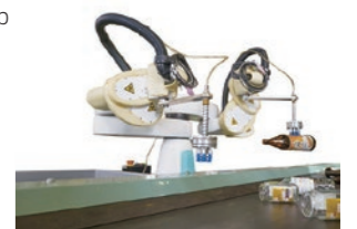
K-Repos AI-equipped resource sorting support system
