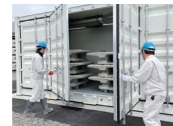
A CO 2 -SUICOM carbonation curing chamber
