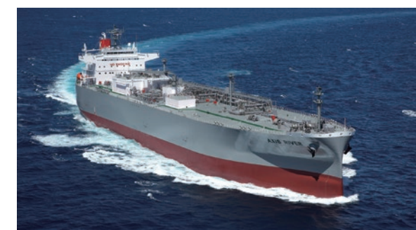
86,700 m 3 LPG-fueled LPG/ammonia carrier
