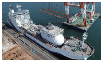
Installation of liquefied hydrogen tank for marine transport
