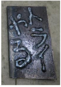
A steel plate with text formed through semi-automatic arc welding
