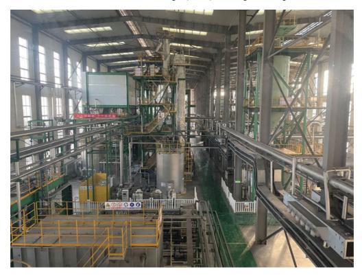
The "Lithium Ion Battery (LIB) Recycle System" is a system that recovers rare metals from used automotive LIBs with high efficiency and low environmental impact. The rare metals contained in automotive LIBs are recycled, and highly efficient lithium recovery is made possible by improving energy efficiency, such as by using exhaust gas from cement manufacturing facilities from the preliminary roasting to roasting process.
