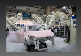
■ Reduced arm weight cuts power consumption by more than 20% compared with existing models
