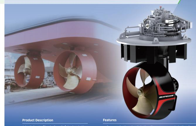
Azimuth thruster "E-series Rexpeller" developed with the "three Es" as its key concepts: Energy saving by improving propulsion performance; Easy maintenance inside the ship; and Environmentally friendly.
