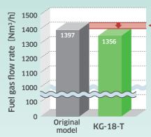
Reducing 41Nm<sup>3</sup>/h = 3% of fuel gas flow rate
