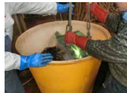
Figure 4: After improvement: Removal of resin using solvents
