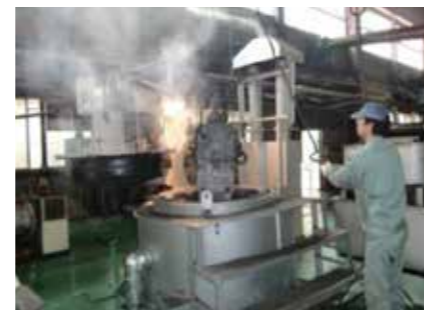
Figure 3: Before improvement: Heating incineration of resin
