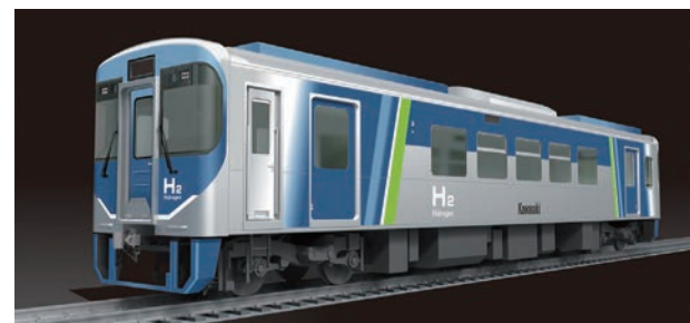
GreenHICE Car, hydrogen-ready train car to replace a diesel engine car
