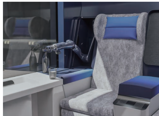
Support provided by the robotic arm mounted on the side of the seat
