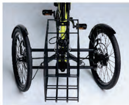
(a) Link structure in which the wheels tilt in line with the body's lean
