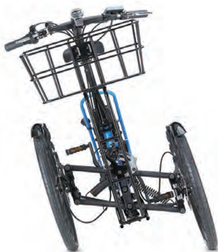
(a) Link structure in which the wheels tilt in line with the body's lean
