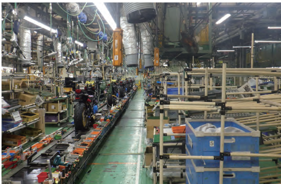
Fig. 1 Lineside parts racks and the poka-yoke system
