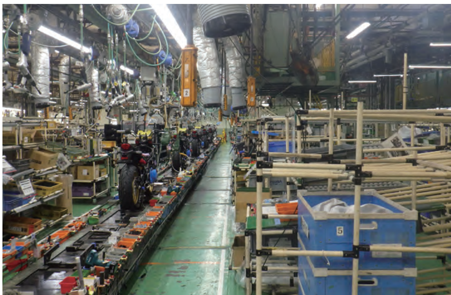
Fig. 1 Lineside parts racks and the poka-yoke system
