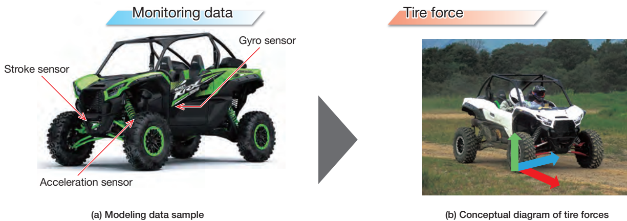
Fig. 4 Measurement method of the tire force 2)
