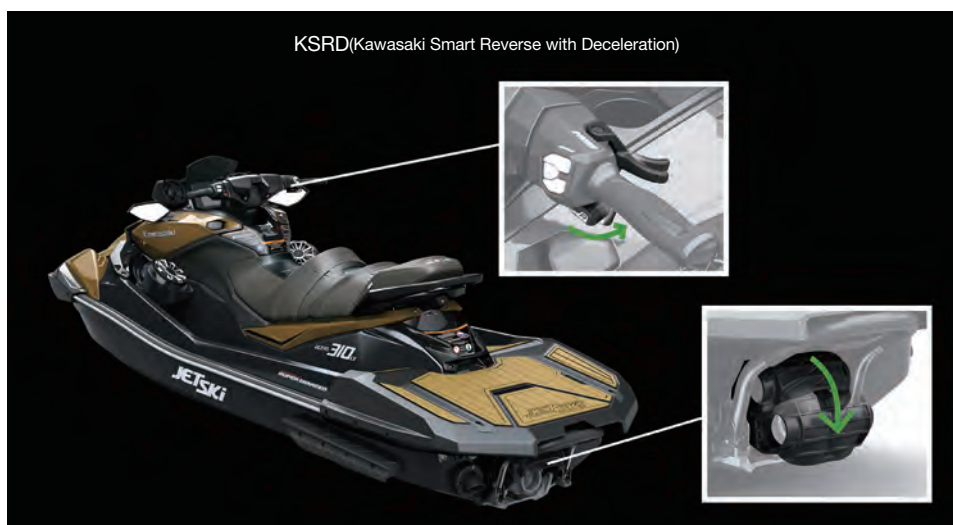
Fig. 2 Image of KSRD system
