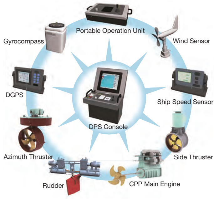
Fig. 4 Example of system construction of KICS-5000
