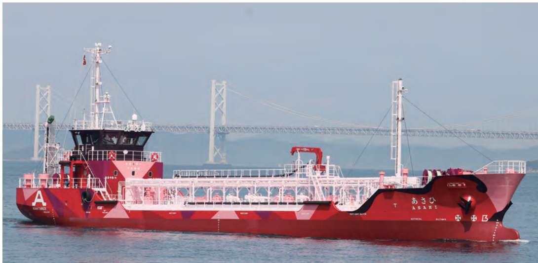
Fig. 3 Pure battery tanker Asahi
