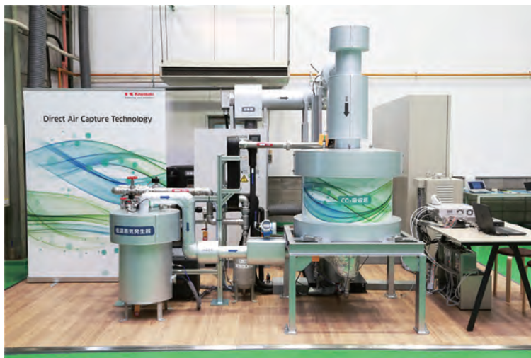
Fig. 6 Demonstration plant for DAC
