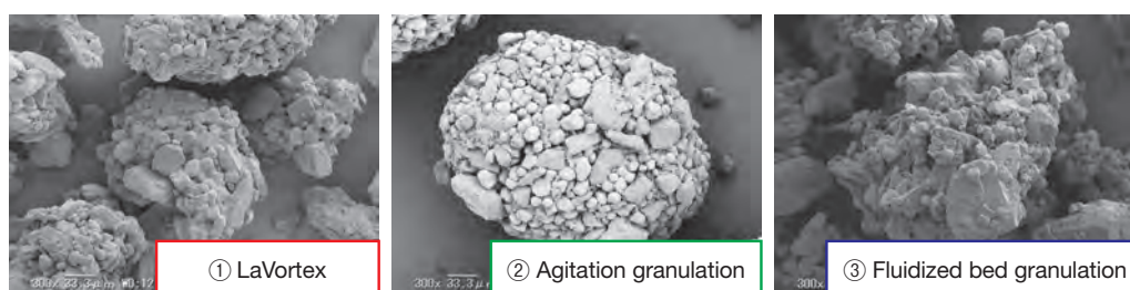
Fig. 3 Granular shape and surface condition
