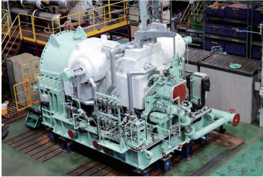
Fig. 2 Steam turbine (for power generation)
