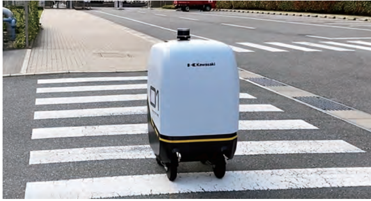
Fig. 4 Demonstration test on a factory road of the first prototype on a factory road
