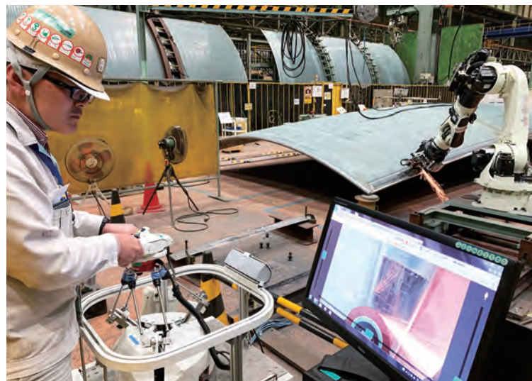
Fig. 5 Grinding operation using Successor-G
