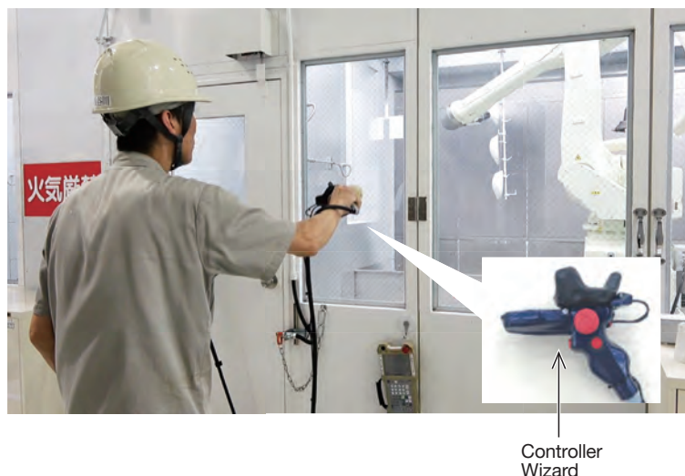
Fig. 4 Painting operation using Successor adapted for coating
