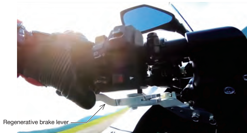
Fig. 7 Regenerative brake operation
