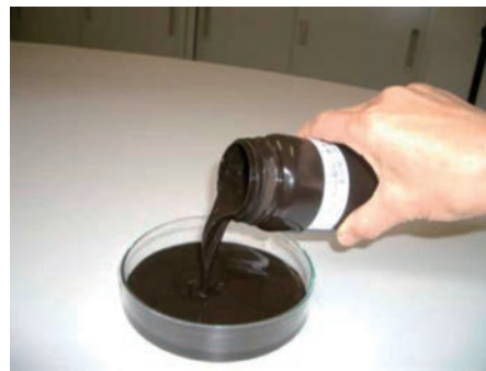
(b) Brown-coal slurry
