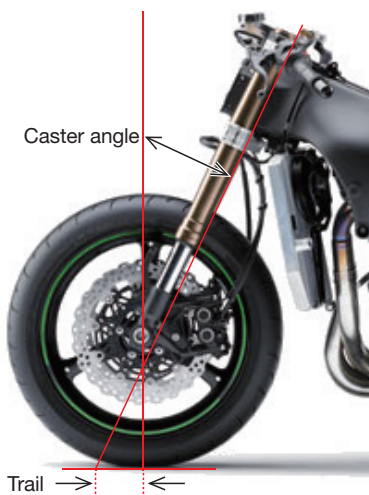
Fig. 1 Caster angle and trail
