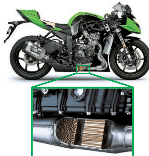
Fig. 8 Three-way catalyst for motorcycle (Honeycomb form)
