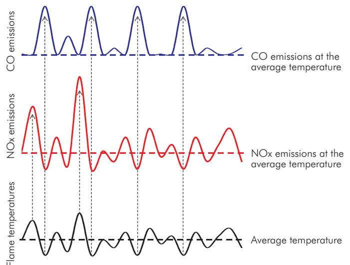
Fig. 1 Relationship between NO<sub>x</sub> and CO formations and flame temperature distribution
