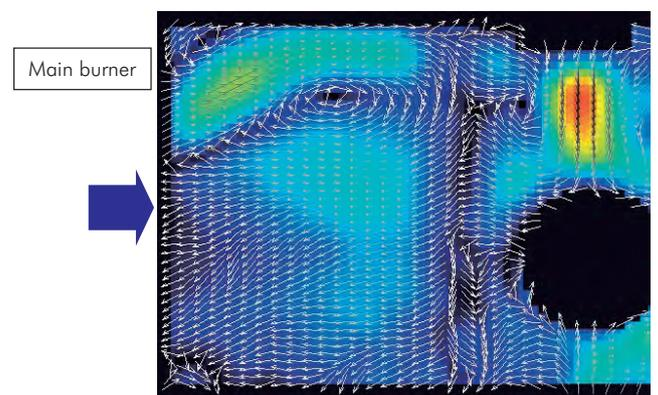
Fig. 8 Result of PIV measurement (Velocity vector)
