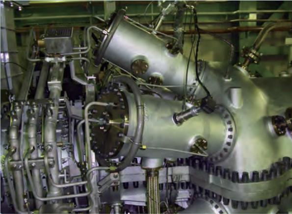
*With a product lineup of 0.7 to 30 MW class gas turbines, we are engaged in the development of combustors and working to commercialize them with the aim of assuring the world's top class emission performance in all models. This paper describes the development and demonstration of Kawasaki's DLE (Dry Low Emissions) combustion technologies.*
