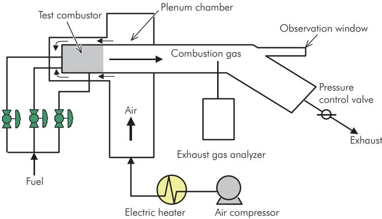
Fig. 9 System diagram of combustion test facility
