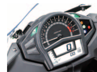
Multifunction LCD meter
