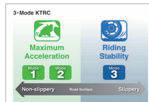
Operational modes of Kawasaki TRaction Control
