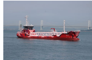
World's first pure battery tanker, ASAHI (Photo by Asahi Tanker Co., Ltd. & e5 lab)
